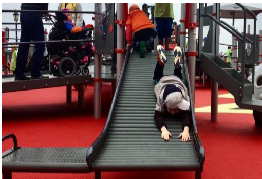
Roller slides provide a tactile and auditory experience. For kids with cochlear implants, it eliminates static.
