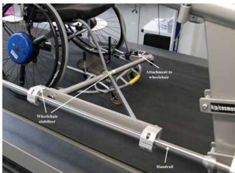
Illustration of the experimental set-up used during the treadmill testing, with the instrumented SMARTWheel attached to determine propulsion kinetics.
